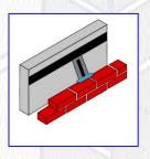
In brick/block situations where the cavity tray is being built into both the inner and outer leaf, the tray is sandwiched within the mortar joints on each course. Where joints are formed in the linear run, a joint support should be used to allow positive forming of the joint which is left in as part of the system.
